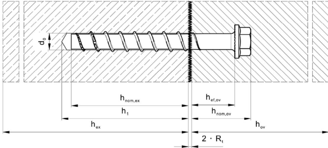
$h_{nom,ex}$  Overall embedment depth in existing concrete
