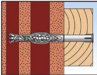
5. Correctly installed anchor in hollow masonry.
