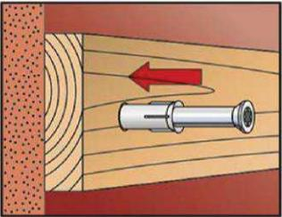
3. Insert anchor (screw and plug) by using a hammer until the collar of the plastic sleeve is flush with the surface of the fixture.
