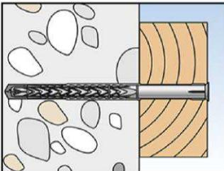
6. Correctly installed anchor in concrete.
