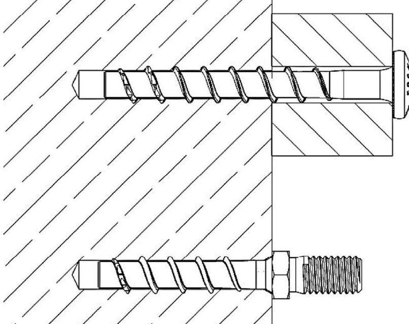
Installed condition in prestressed hollow core slabs
