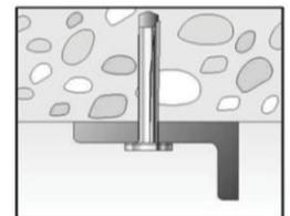
4: Installed fastener
