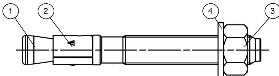
Cone bolt manufactured by turning:
