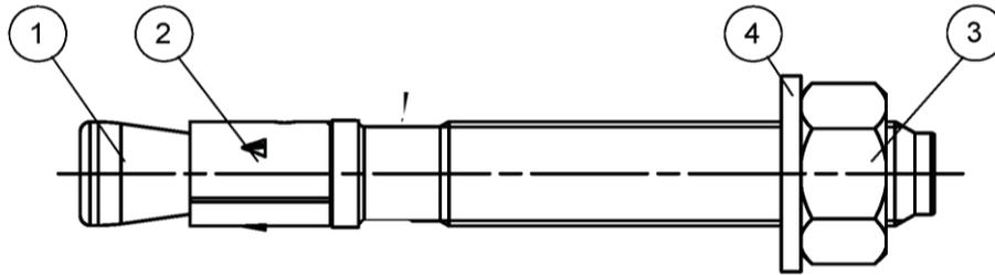
Cone bolt manufactured by turning:
